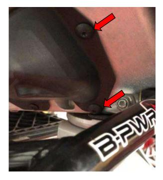
4.12 Loosen the 2 lock nuts that hold the steering rod and completely unscrew the steering column
