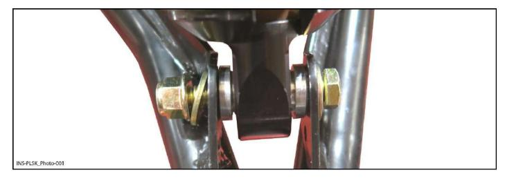
3.2 Remove and discard screw located in middle of leg retaining stabilizer bar.
