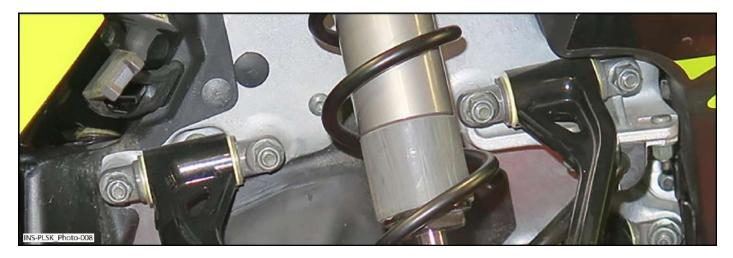
3.6 Hold one end of OEM arm and using snap-ring pliers remove retaining ring that holds pivot in place. Remove and keep washers, retaining ring and pivot.
