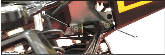
Front section shown 1- Screw that goes through chassis 2- Nut
