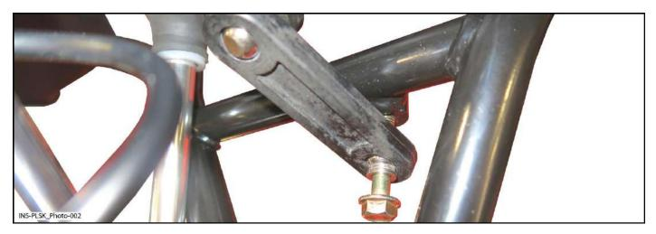
3.3 Remove and keep the screw, nut and washers. Start with lower one to provide access to upper nut. Remove upper nut and remove arms from ski leg.
