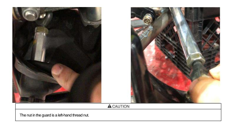
4.13 Slide the steering rods [P12] into the protectors and screw them to the two ball joints respectively.
