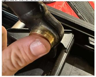
4.7 Once the brass is pressed in fully, install the retaining ring included in your kit. If the retaining ring does not seat fully in the groove, the brass is most likely not pressed in fully. Repeat step 4.6 to get the brass fully seated.
