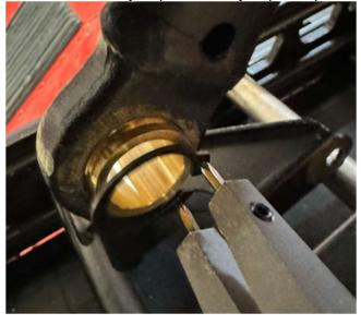
4.8 Install the stainless sleeve from your kit into the brass piece, and then reinstall the rear swing arm back into the triangle bracket.
