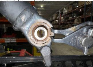
4.5 Using a C clamp and two socket (15mm & 22mm), pressed out the heim joint.
