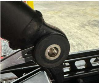
4.4 Using a pair of snap ring pliers, remove the internal retaining ring holding the heim joint in.
