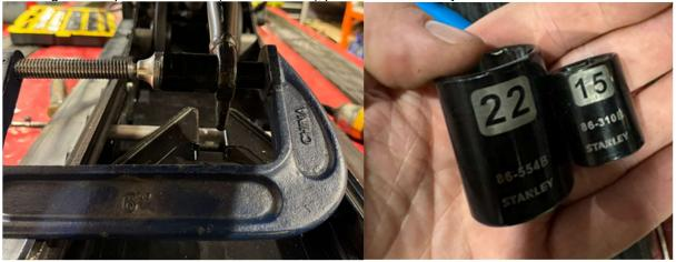
4.6 Once the heim joint is removed, install the brass bushing from your delete kit in it's place, snap ring groove first. Try to push it in and line it up the best you can by hand first. Then, using a C clamp, press the brass in as straight as you can. Be very careful to press the brass in evenly. DO NOT HAMMER DIRECTLY AGAINST THE BRASS. The brass is very soft and will deform if hammered directly against, or with an uneven punch.
