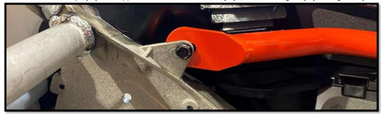
4.4 Secure the G5 front bumper [P1] with four (4) 3/16" rivets [P4] using a hand riveter.
