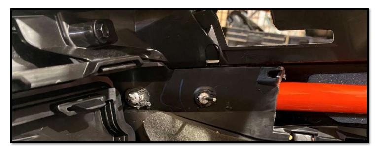
4.5 Tighten to the specified torque two (2) M6 self-locking nuts [P3].
