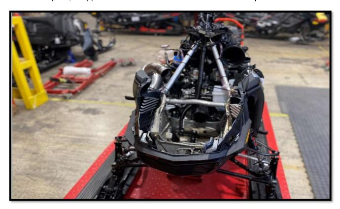
4.2 Remove the existing bumper. Drill the rivets using a 3/8" dia drill bit. Take the necessary precautions to avoid damaging the plastic of the bodywork.
