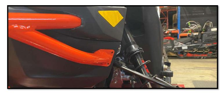
4.5 Secure the G5 front bumper [P1] with four (4) 3/16" rivets [P4] using a hand riveter.
