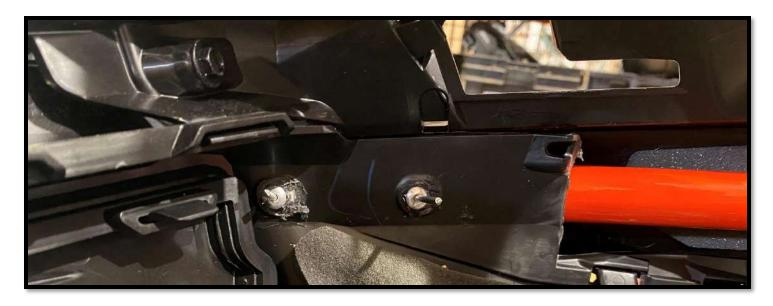
4.6 Meter in place the bracket for the muffler temperature switch.
