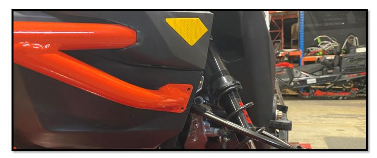
4.5 Secure the G5 front bumper with four (4) 3/16" rivets using a hand riveter.
