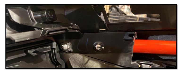
4.6 Insert in place the muffler temperature switch bracket.
