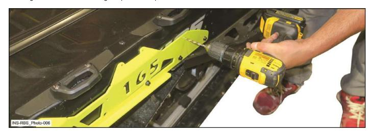
4.5 Secure bumper with 3/16" rivet [P2] in previously drilled holes as shown.
