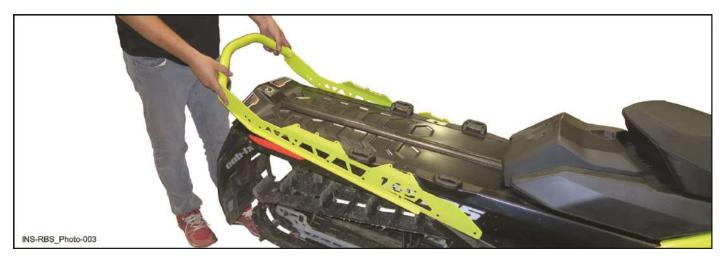
4.2 Install rear bumper [P1] with M6 X 20 mm hexagonal flanged screw [P3] and M6 nylon lock nut [P4].
