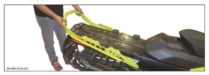
4.2 Install rear bumper [P1] with M6 X 20 mm hexagonal flanged screw [P4], one (1) M6 X 16 mm hexagonal flanged screw [P3] at front of vehicle and M6 nylon lock nut [P2].
