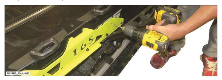
5.5 Secure bumper with 3/16" rivet [P5] in previously drilled holes as shown.
