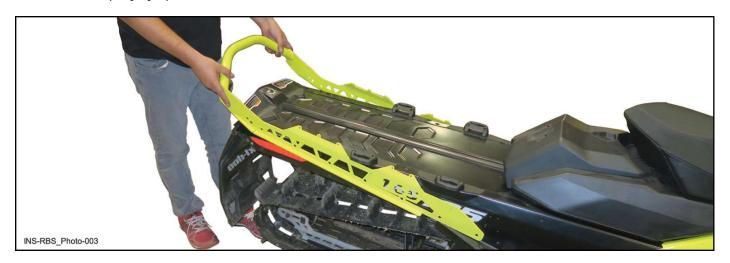
4.2 Install rear bumper [P1] with M6 X 20 mm hexagonal flanged screw [P2] and M6 nylon lock nut [P3].
