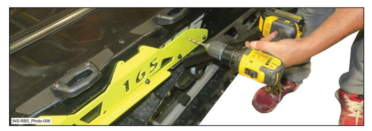
4.5 Secure bumper with 3/16" rivet [P4] in previously drilled holes as shown.
