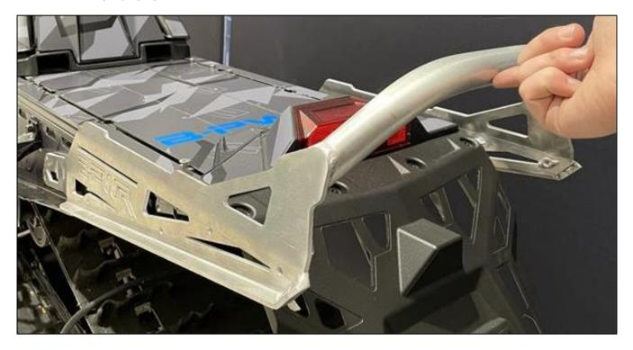
4.4 Locate rear bumper [P1] with flanged hex head screw [P2], flat washer [P5], and lock nut [P3]. Hand tighten only.
