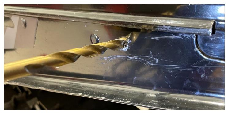
4.1 With the help of a drill and a 5/16" drill bit, remove the existing rivets, as shown below.
