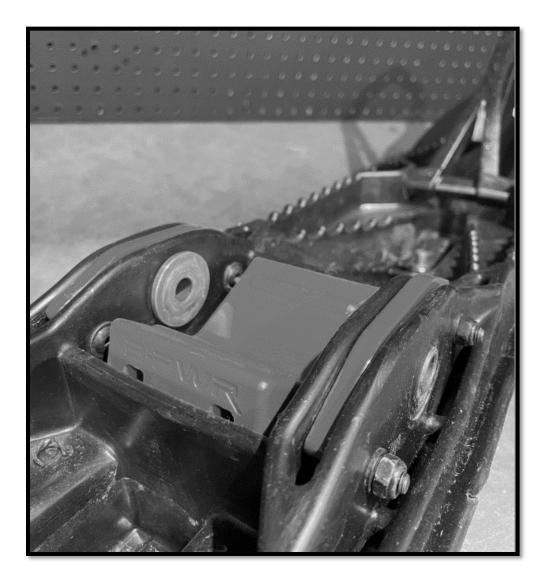
3.2 Reinstall your ski on the snowmobile. Make sure to reuse the OEM bolts and nuts in the assembly. Tighten the nut to the builder's specifications.
