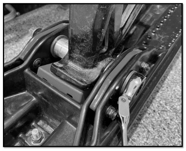
3.3 Repeat steps 3.1 and 3.2 for the second ski rubber. Don't forget to tighten the bolts and nuts.
