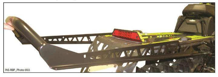
4.2 Locate rear bumper [P1] with M6 X 20 mm hexagonal flanged screw [P3] and M6 nylon lock nut [P2]. Hand tighten only.
