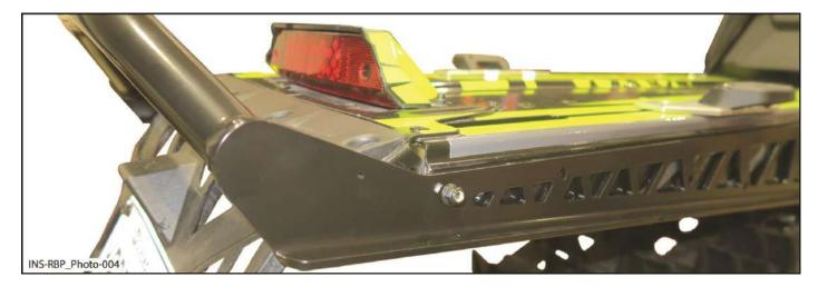
4.6 Secure rear of bumper with M6 X 16 mm hexagonal flange screw [P3] and M6 nylon lock nut [P2] in previously drilled holes as shown. Tighten to specification.
