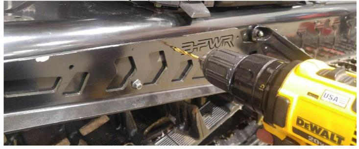
4.5 Secure front of bumper with 3/16" rivets [P4] in previously drilled holes as shown and using hand riveter.
