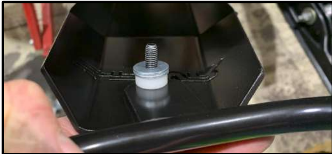
4.4.3 Light Duty without Skidplate Note : 1X Washer [P5] and 1x Washer [P7]
