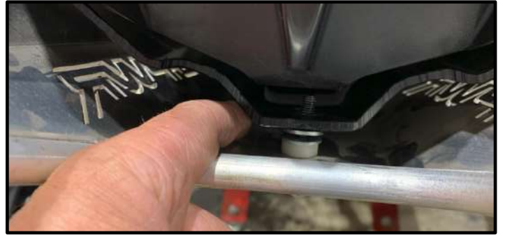
4.4.2 Heavy Duty with Skidplate Note : 1x Washer [P5] and 1x Washer [P7]
