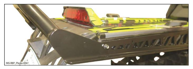
4.3. Drill holes in front of the tunnel using bumper as a template with drill bit 3/16" as shown.
