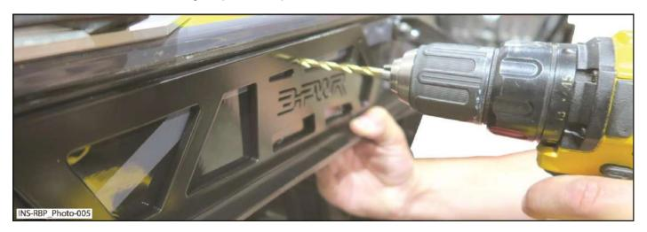
4.4 Secure front of bumper with 3/16" rivets [P5] [P6] in previously drilled holes as shown and using hand riveter.
