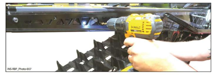
4.6 Secure rear of bumper with M6 X 16 mm hexagonal flange screw [P4] and M6 nylon lock nut [P2] in previously drilled holes as shown. Tighten to specification.
