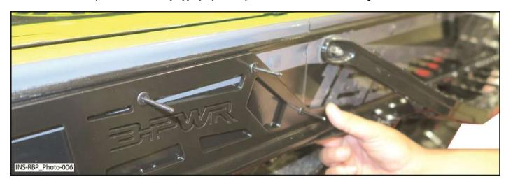
4.5 Drill holes in tunnel using bumper as a template with drill bit 1/4" as shown.
