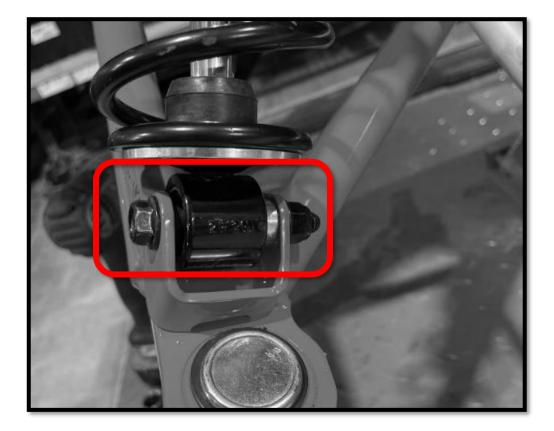
3.7 Repeat step 3.1 for the upper control arm [P3] or [P4]. Once the OEM spacers and bushings are installed in the control arm, insert your two bolts and four washers. See picture below for more details.
