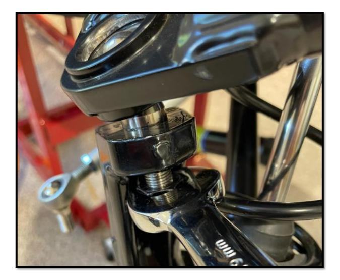
3.12 Reinstall your ski. Don't forget the ski rubber that goes between the spindle and the ski. See picture below for more details.
