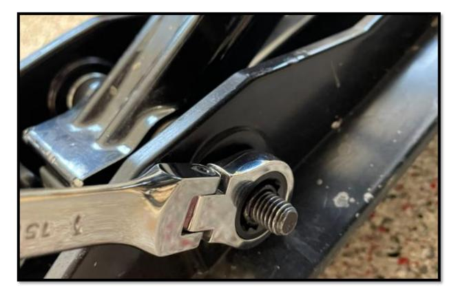
3.14 install the tie rod end in the spindle.
