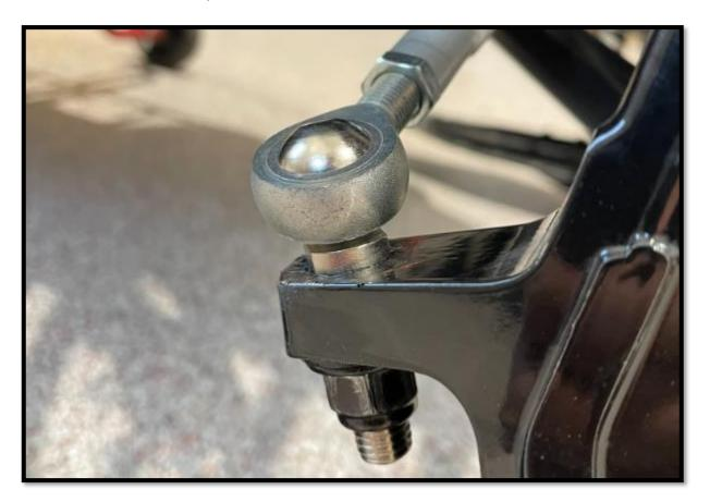
3.13 Tighten the nuts and bolts to the manufacture's specs. At the point, it is possible that an ajustement is required in your steering alignement. Follow the manufacturer recommendations for this step. End of installation.
