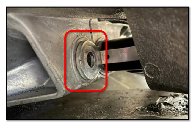
3.4 Once to lower control arm [P1] or [P2] is in place, reinstall all your nuts and bolts. Make sure to discared of the old elastic nut and use the new nuts included in your B-PWR kit. See picture below for more details.
