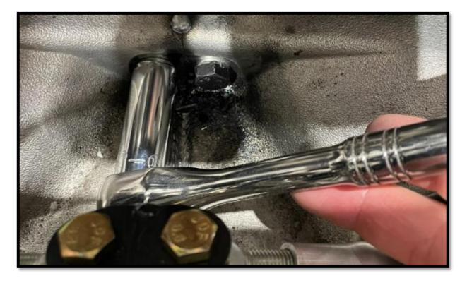
3.6 Put the shock and swaybar back in their place, reinstall all your nuts and bolts. Make sure to discared of the old elastic nut and use the new nuts included in your B-PWR kit. See picture below for more details.
