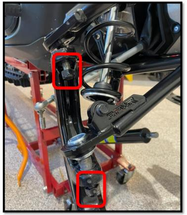
3.11 Tighten the nuts and bolts to the manufacture's specs.
