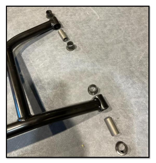
3.3 Once the bushing are inserted in your lower control arm [P1] or [P2], you can now install your lower control arm [P1] or [P2] on the machine. Pay special attention to the spacer plate included with the snowmobile, it must be aligned with the axis of the control arm's bushing during the installation. See picture below for more details.
