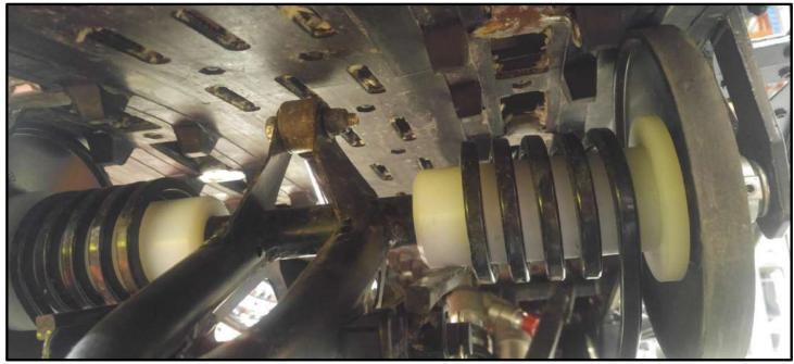
$4.5\,$  Re-install the wheel, spacer and small screwRemonter la roue, l'espaceur et la vis à 6 pan creux (see vehicle user manual for tightening torque). Lower the back of the snowmobile.
