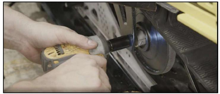
4.7 List the rear os the snowmobile, replace the spring forward (tension) and replace the spring support.Remonter le derière de la motoneige, remettre le ressort vers l'avant (en tension) et remettre le support (see vehicle user manual for tightening torque)
