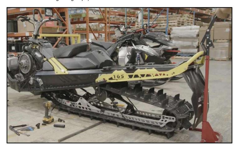
4.6 Adjust the position with the help of a bar to lift the rail, and insert the hex bolt. (see vehicle user manual for tightening torque)
