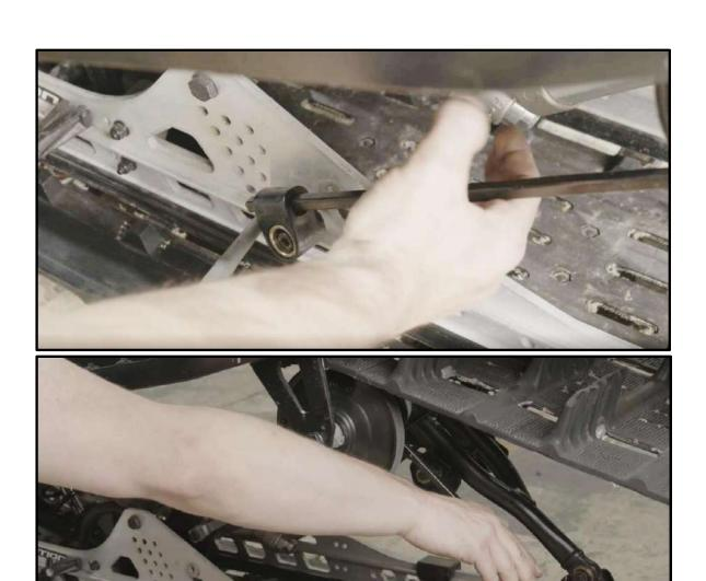
4.3 Unscrew the hex bolt and small screw to remove the spacer and wheel.
