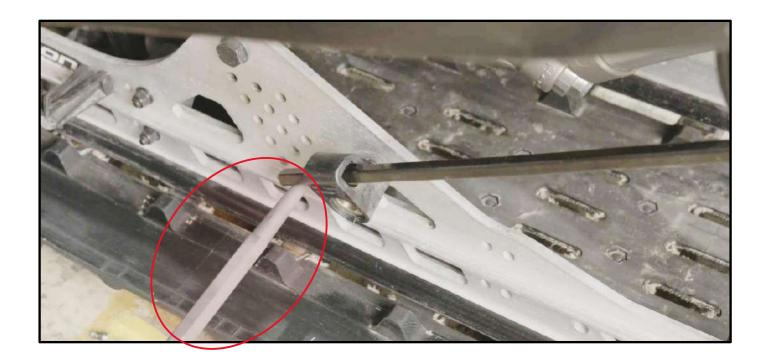
$4.2\,$  Unscrew the screw of the spring support piece, while holding the spring. Once unscrewed place the spring towards the rear of the vehicle.
