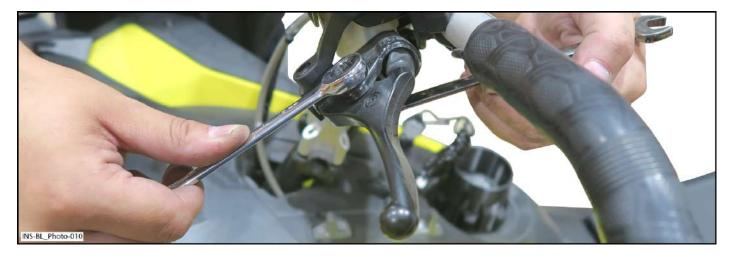
4.2 Remove and keep E clip and dowel pin holding brake holder with a flat screwdriver [T1].
