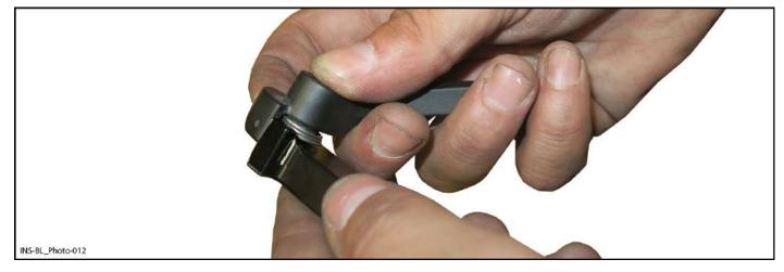
5.2 Secure brake holder on aluminum brake lever [P1] with E clip previously removed using a flat screwdriver [T1].
