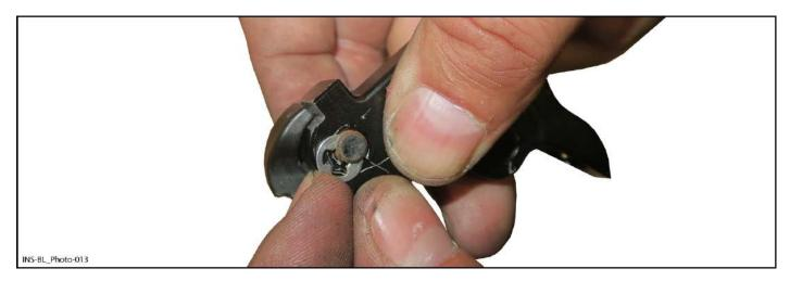
5.7 Secure aluminum brake lever [P2] using two (2) 10 mm wrench key [T4].
