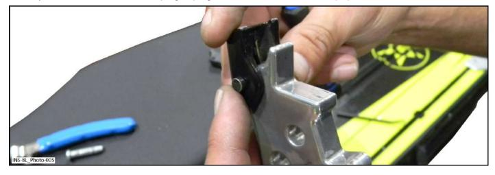
5.2 Secure brake holder on aluminum brake lever [P1] with push nut.
