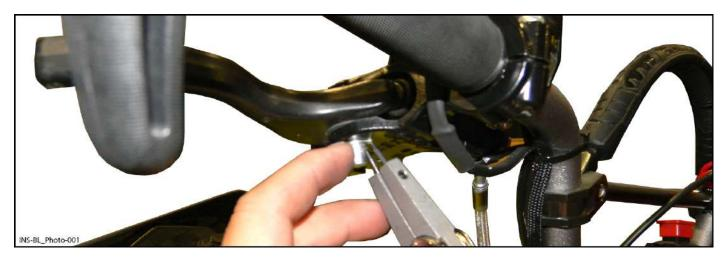
4.2 Remove and keep dowel pin as shown.
