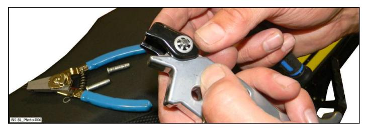
5.3 Install aluminum brake lever [P1] with dowel pin previously removed.
