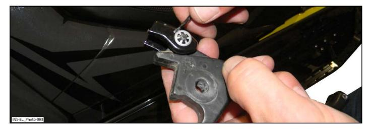
4.4 Remove brake holder and keep spring in same position.
