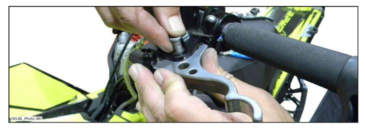
5.4 Secure aluminum brake lever [P1] by inserting snap ring into dowel pin groove using snap-ring pliers [T2] as shown.
