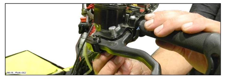
4.3 Remove and keep push nut and dowel pin holding brake holder with a flat screwdriver [T1].
