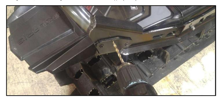
4.8 Install screw [P10] into the drilled hole, and hand-tighten nut [P11] onto it.
