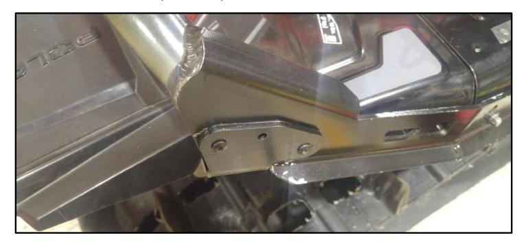
4.7 Using a 3/16" bit, drill a hole through the center hole of each lateral support [P4 - P5].
