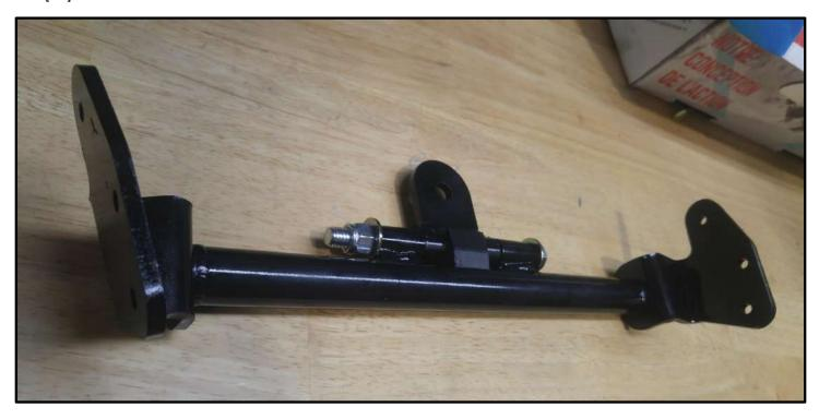
4.6 Align the hitch attachment with the holes in the bumper and install 2 M5 screws [P10] through the lateral supports and number; handtighten.
