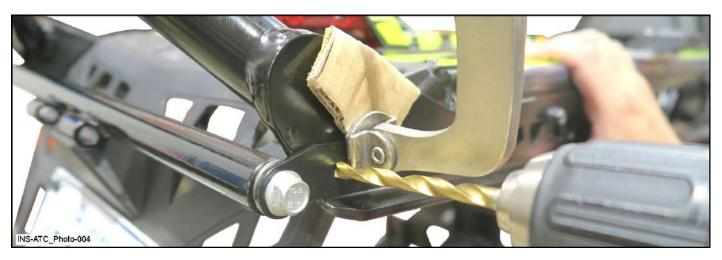
$3.5\, \text{Remove Tube with nut BRP / Polaris [P1] drill one (1) hole in bumper using mark made earlier as shown.}$
