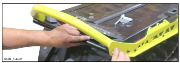
4.14 Secure Tube with nut BRP / Polaris [P1] on bumper with two (2) using wrench key.
