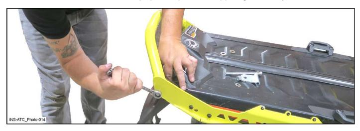
4.15 Install Languette [P2] with two (1) Washer 3/8 [P6], 3/8 - 16 X 4 3/4" Partially Threaded 1" [P3] and Lock Nuts - 3/8 - 16 - Nylon [P4].
