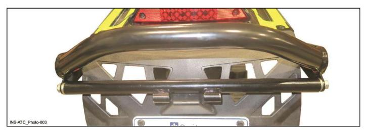
3.4 Secure Tube with nut BRP / Polaris [P1] with locking c-clamp and mark one (1) hole in bumper using ATC 3 trous Bracket - holes bracket [P8] as a template with drill bit 3/16" as shown.
