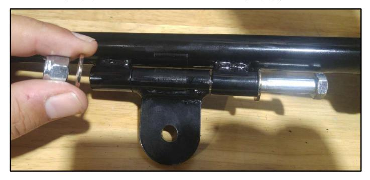
3.9 Secure Languette [P2] with two (2) 9/16" wrench key.
