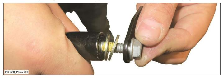
3.2 Position Tube with nut BRP / Polaris [P1] on rear bumper as shown.
