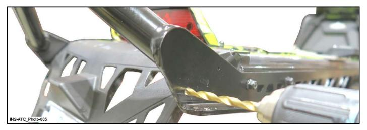
3.6 Secure ATC 2 trous Bracket [P7] on Tube with nut BRP / Polaris [P1] with Hex Head Cap Screw - M6 - 1X20 MM - Fully Threaded [P9], Lock Nuts - Flanged - M6 - Nylon [P10] and drill one (1) hole in bumper using ATC 2 trous Bracket [P7] as a template with drill bit 3/16" as shown.
