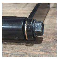
4.9. Position the tube at the height and torque to the specified torque.
