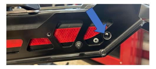
4.32 Using the B-PWR bumper rivet hole as a guide, drill the tunnel with a 9/32' drill.
