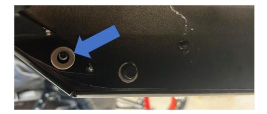
4.5 Insert the lateral support plate [P1] on the screws [P2]. Insert the nuts [P3] on the screws [P2]. Tighten to the specified torque.
