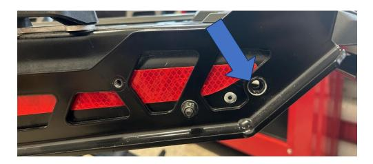
4.32 Using the B-PWR bumper rivet hole as a guide, drill the tunnel with a  $9/32^{\prime}$  drill.
