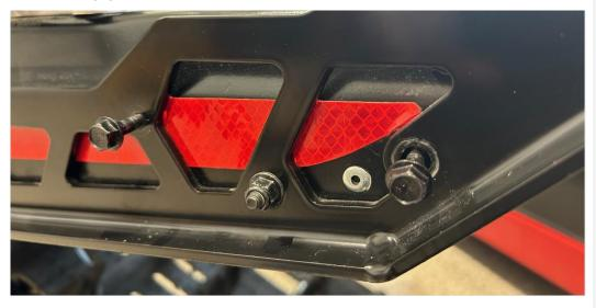
4.4 Inside the tunnel, insert the washer [P6] on the screw [P2] furthest back of the tunnel.
