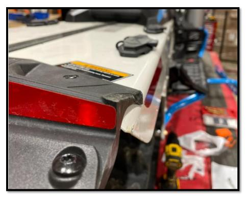
4.2 Once the snow flap has been trimmed, dispose of the nylon lock nut used to hold the rear of the foot boards. You will find 4 screw and 2 lock nuts on each side of the machine. (See pictures below for more information).
