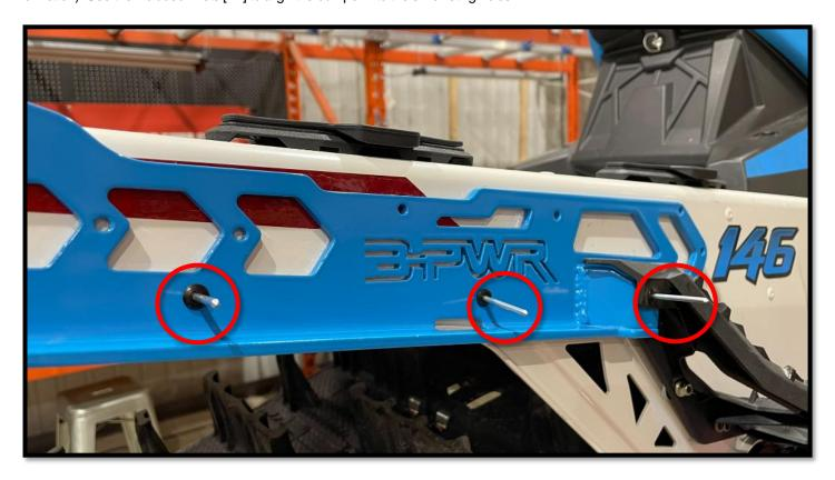
4.4 Once the rivets went into place, make sure to fasten them accordingly with the rear bumper [P1] and the tunnel.
