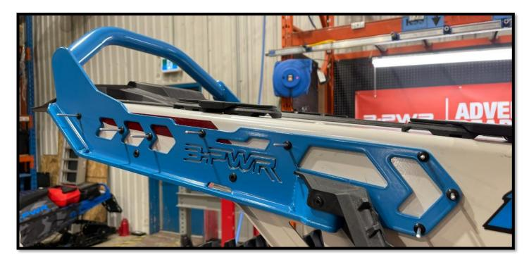
4.8 Rivet the entirety of the bumper [P1] and tunnel together.
