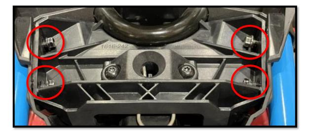
$4.9\,\mbox{Tighten}$  the four screws [P4] to the builder's specifications.
