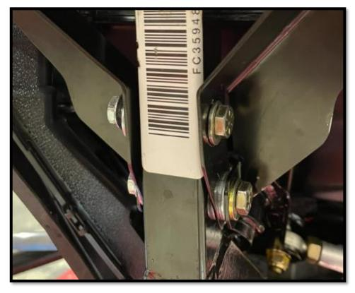
4.4 Align the front brace plates with the already existing upper holes in the snowmobile's frame. The top face of the plates should line up with the top of the snowmobile's plastic frame. (See picture below for more details).
