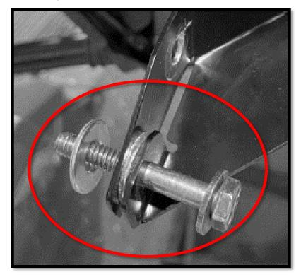
4.3 Install both front braces on the snowmobile. Pay attention to the washer installation sequence, as a wrong sequence will result in an unproper installation. One both braces and hardware installed, only hand tighten the  $\frac{1}{4}$ -20 nuts [P7] included in the hardware kit.
