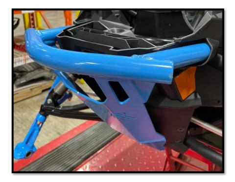
4.8 Install the four flanged hex screw [P4]. Do nut fully tighten them until threads are engaged on all four corners.
