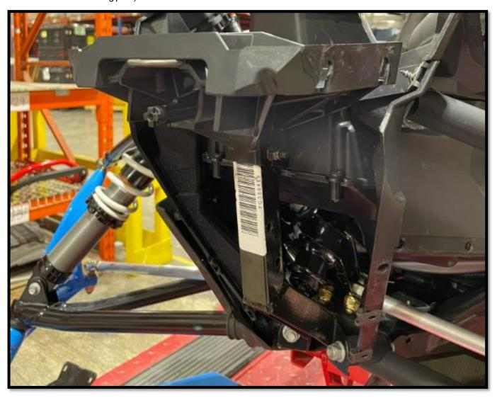
4.2 Once the front skid-plate has been removed, take your front braces [P2] and [P3] and insert a flat washer [P8] in each brace. Preassemble your hardware as shown in the picture below.
