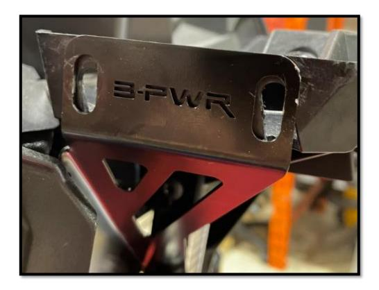
4.5 Once the plates properly aligned, tighten both  $\frac{1}{4}$ -20 nuts [P7] to the builder's specifications.
