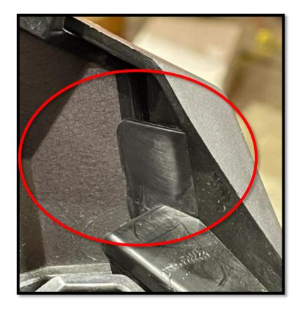
4.7 Once all the skid-plate hardware is reinstalled, insert the front bumper [P1].
